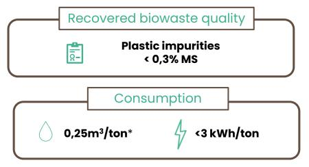
\*The bio-SV does not require the addition of water to operate. It is possible to add dirty water to limit water consumption.
